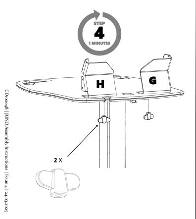
Place both retainers (H+G) into the slots\* and fix using wing nuts provided. If the laptop is to be fitted later, leave loose so the retainers can be easily moved for laptop installation.
