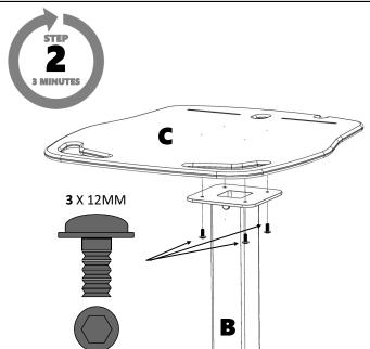
Insert and tighten the (BLACK) 3 x 12MM flange head fixings through the central column (B) into the work surface (C)
