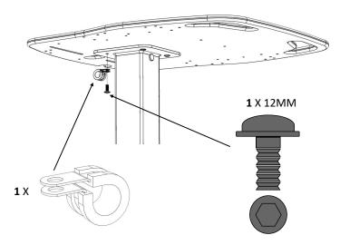
Insert and tighten the (BLACK) 1 x 12MM flange head fixings through P-clip then central column (B) into the work surface (C)
