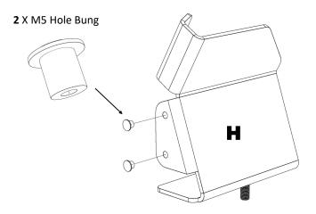
Insert 2x hole bung to both LH & RH retainer (H & G) (If using accessory holders miss step)
