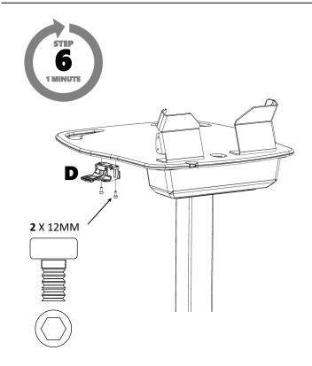
Attach the height adjustment handle (D) using the 2 x 12mm pan head fixings  $\,$
